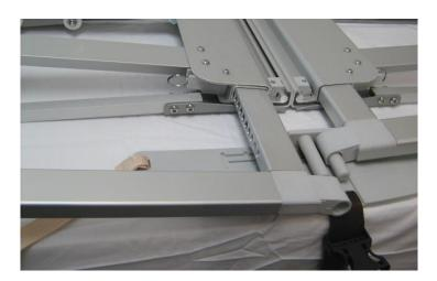
4. Extend the trombone past the strap bracket, then retract the trombone so that it locates correctly on the strap bracket. Engage the trombone locking pin. Repeat for the other side of the bed.
